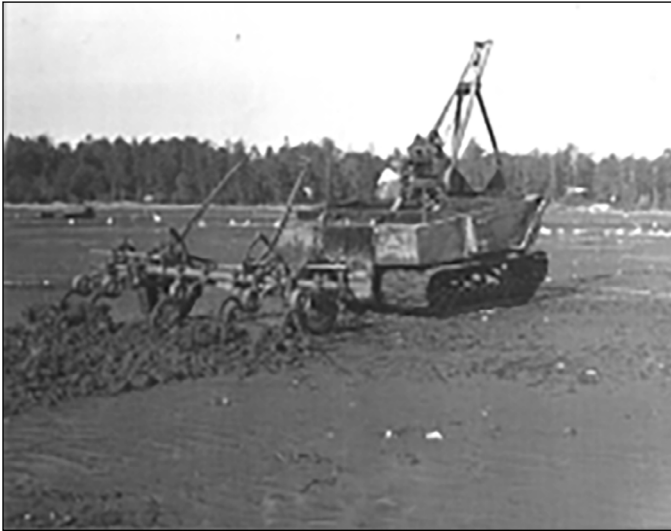
Figure 4. Weasel pulling a spring tooth harrow across an oyster bed. Photo courtesy of Dennis Tufts.
