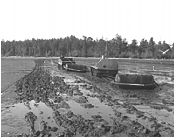
Figure 6. Weasel (in lead) and Snow Cat pulling rollers. Photo courtesy of Dennis Tufts.
