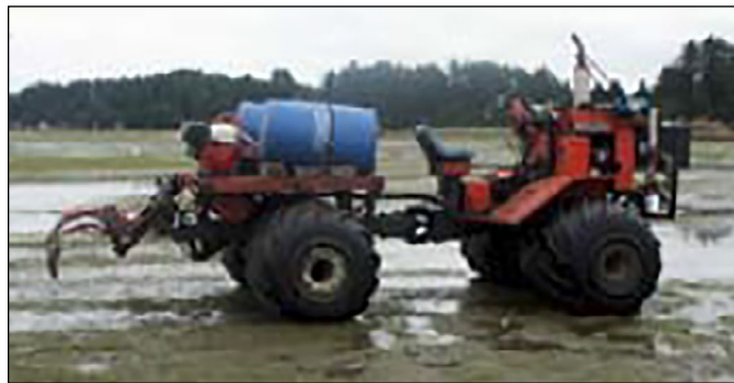
Figure 13. A Rolligon modified to inject chemical controls. Photo courtesy of Steve Booth.
